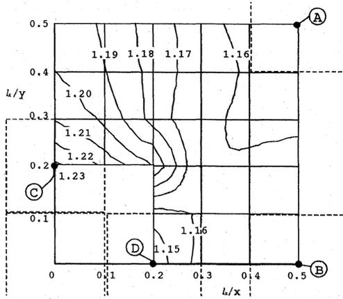
Fig. 7.  $E/E_M$  vs. central coordinate of inclusion  $B$  in model (1) ( $b/a = 1, ab/l_x l_y = 0.08, E_I/E_M = 10^5$ ).
