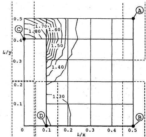
Fig. 9.  $E/E_M$  vs. central coordinate of inclusion  $B$  in model (3) ( $b/a = 4, ab/l_x l_y = 0.08, E_I/E_M = 10^5$ ).
