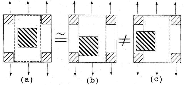
Fig. 10. Elastic modulus is almost equal in (a) and (b), but not equal to (c).
