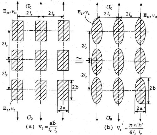
Fig. 4. Elastic modulus is almost equal when. (1)  $a = a'$  and (2)  $ab = \pi a' b' / 4$ .
