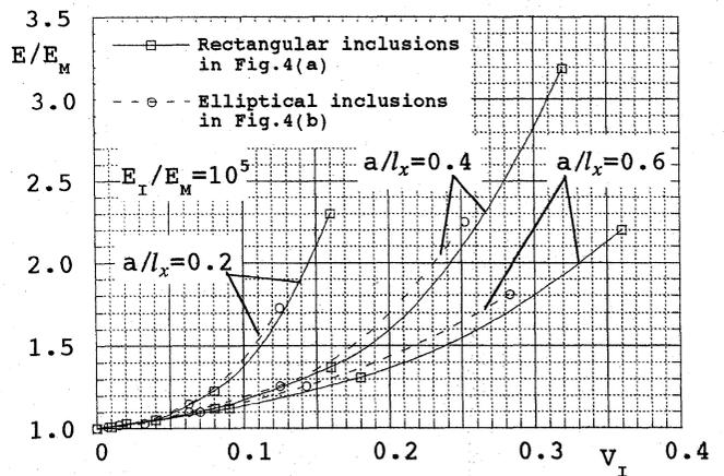
Fig. 3.  $E/E_M$  vs.  $V_I$  relation in Fig. 4<sup>15)</sup>.
