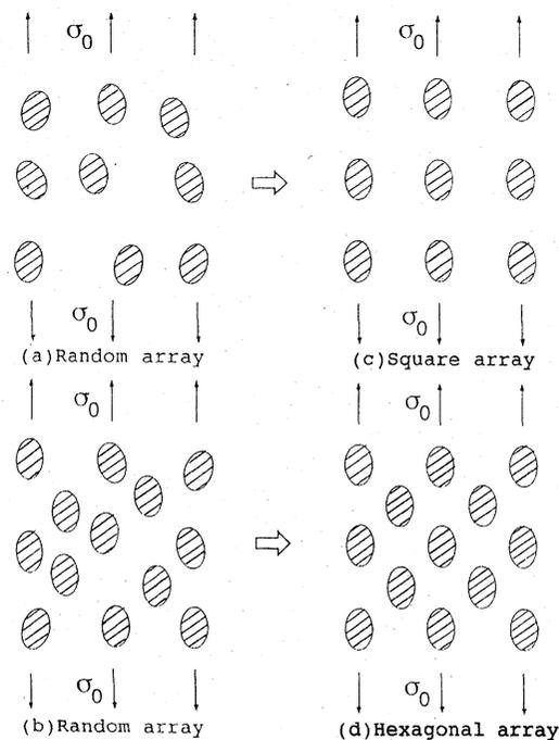
Fig. 1. Periodic arrangement of elliptical inclusions.
